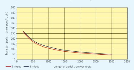
The shorter the route, the higher the performance. For an aerial tramway length of 500 m, the transport capacity is already at 200 persons per hour and direction.
